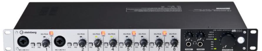
Delivering pristine sound quality, the UR824 audio interface perfectly combines high-speed USB 2.0 connectivity with balanced analog and digital inputs and outputs in various formats. The UR824's front panel hosts two Neutrik combo TRS/XLR connectors for balanced microphone/line input with switchable 48 volt phantom power and Hi-Z, pad push buttons for signal attenuation, gain controls with peak indicators. This
