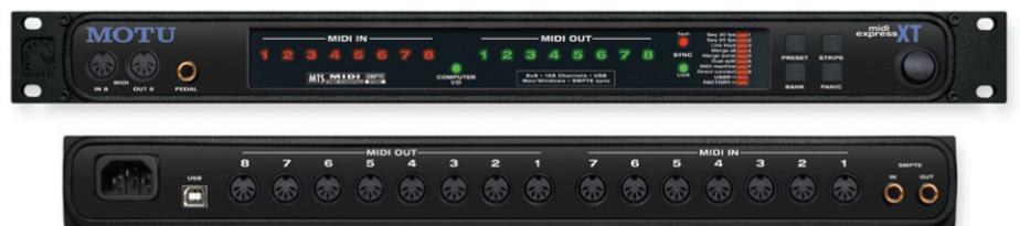
The MIDI Express XT is MOTU's intelligent 128-channel USB MIDI interface for Mac and Windows. You get plug-and-play USB connectivity to any computer, sub-millisecond MIDI timing accuracy, eight separate MIDI inputs, nine MIDI outputs, sync features, a foot switch input, and tons of MIDI processing, including routing, merging, and muting.
